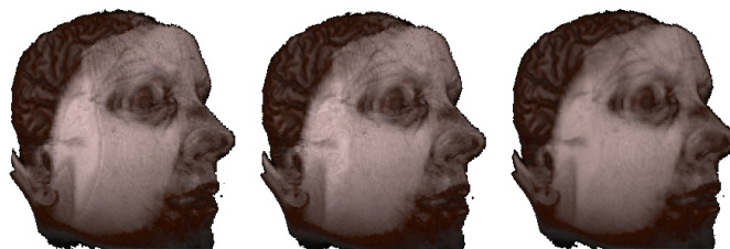
Fig. 3. A volume rendering (left) with stochastic jittering (center) and tri-cubic filtering (right). The stochastic jittering reduces the wood-grain artifacts in the volume, however it is almost imperceptible in this scene. The tri-cubic filtering smooths the volume data, reducing the artifacts present in the volume rendered with trilinear filtering.
